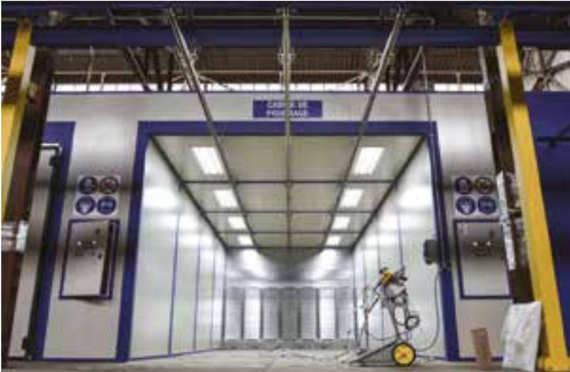
CABINE DE POUDRAGE - ETUVE - DIMENSION STANDARD ET FABRICATION SUR MESURE POSSIBLE
