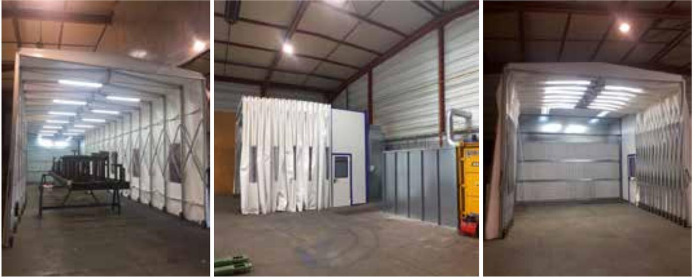
CABINE AVEC AVANCEE RETRACTABLE DE 15 M
