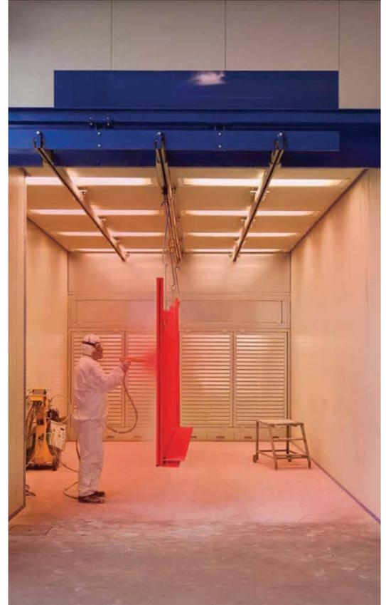
**CABINE DE POUDRAGE - DIMENSION STANDARD ET FABRICATION SUR MESURE POSSIBLE**
